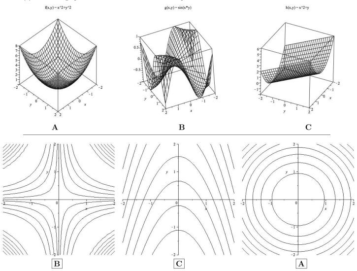
Graph A has the equation  $z = x^2 + y^2$  so its level curves are  $x^2 + y^2 = c$  (circles). Graph B has the equation  $z = \sin(xy)$  so its level curves are  $\sin(xy) = c$  so  $xy = \arcsin(c)$  and thus y = (something)/x which are hyperbolas. Graph C has the equation  $z = x^2 + y$  so its level curves are  $x^2 + y = c$  and thus  $y = -x^2 + c$  (parabolas opening downward).
